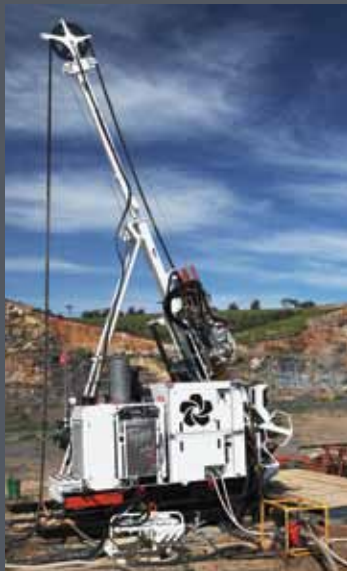
Diamond Coring Rigs
